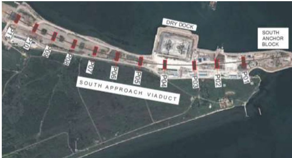
Figure 2. General Layout of South Approach Viaduct Footings
