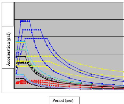
Figure 2. Response spectrum for important bridges [33].
