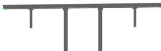
Figure 2. Five span bridge constructed by the incremental launching method.
