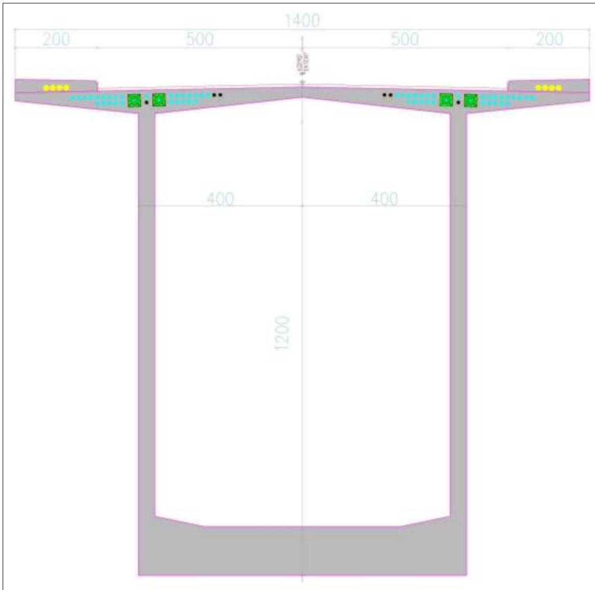
Fig. 7 - Deck Section at The Middle of The Span
