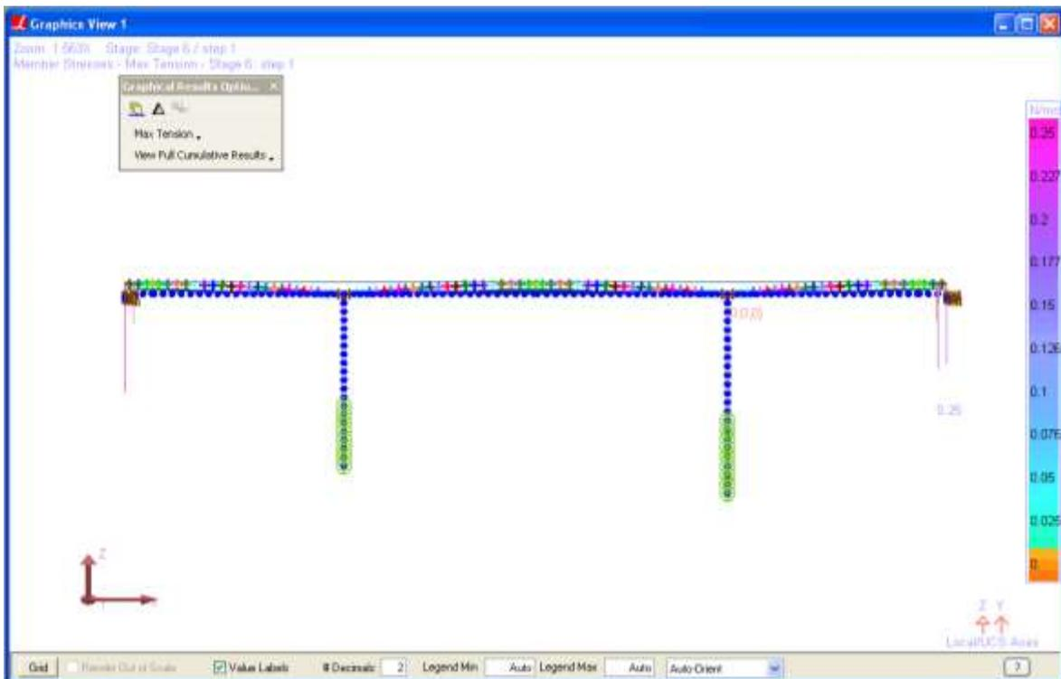
The calculations mentioned above are for the tendon calculations at the top and the bottom of the deck. But during earthquake we have high lateral displacements at the middle of the span and moments at webs of deck at same location. Post tensioning at the webs or using metal plates are the alternatives but they will be hard for the workers to construct. To achieve design limits we used more reinforcement at the middle portions of the spans at the side walls of the deck.
