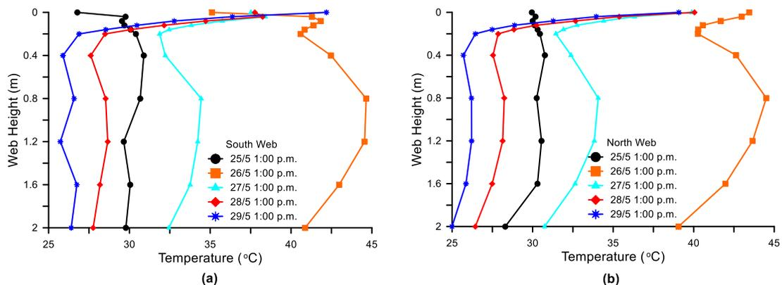
Figure 7 Vertical temperature distributions at 1:00 p.m. for the first five days (a) south web (b) north web
