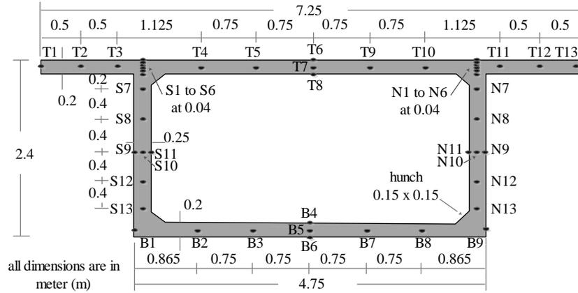
Figure 1 Dimensions of the cross-section of the box-girder segment and the locations of thermocouple
