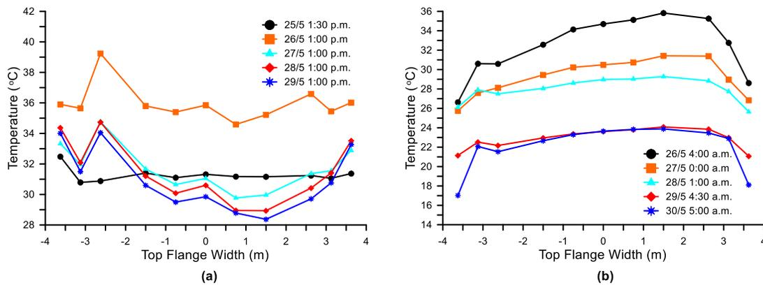
Figure 9 Temperature distributions along the top slab for the first five days (a) afternoon (b) morning
