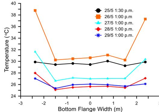
Figure 10 Afternoon temperature distributions along the bottom slab for the first five days
