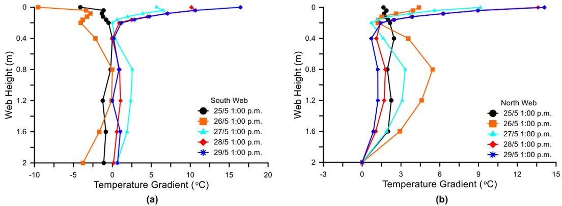
Figure 8 Vertical temperature gradients at 1:00 p.m. for the first five days (a) south web and (b) north web
