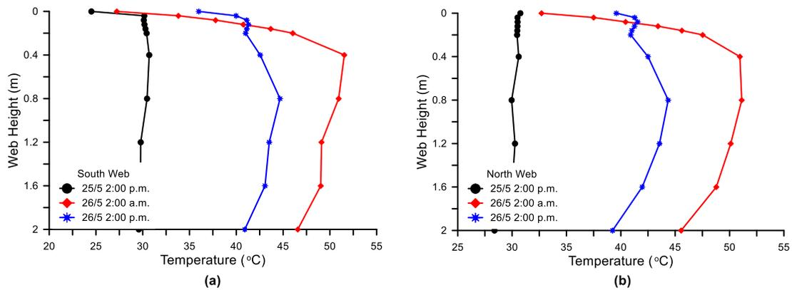
Figure 6 Vertical temperature distributions for selected time steps (a) south web (b) north web
