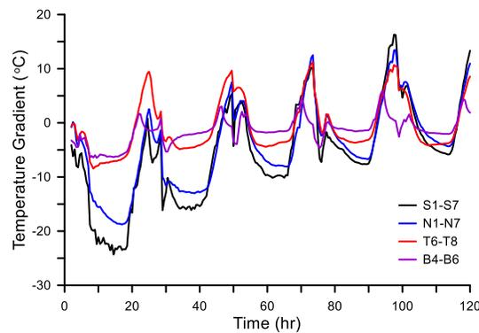
Figure 5 Temperature gradient-time curves for south web (S1-S7), north web (N1-N7), top slab (T6-T8) and bottom slab (B4-B6)
