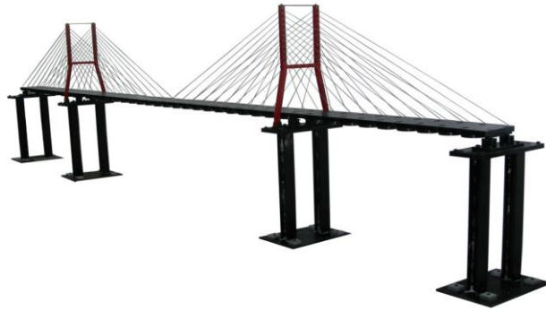
Figure 1. Cable-stayed bridge model
