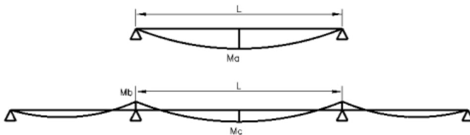
Figure 1. Moment diagram of a simply supported and continuous girder.
