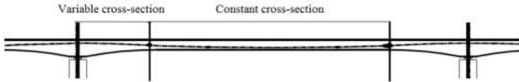
Figure 2. Variable and constant cross-section.
