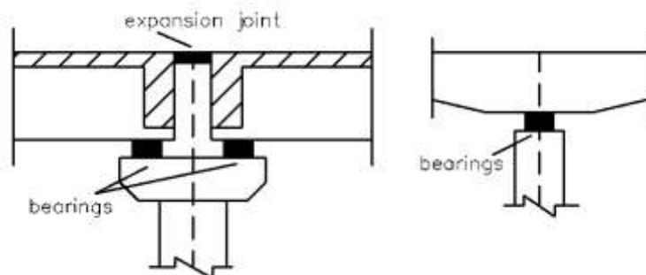
Figure 4. Detail at pier: Precast girder and Continuous post-tensioned girder.
