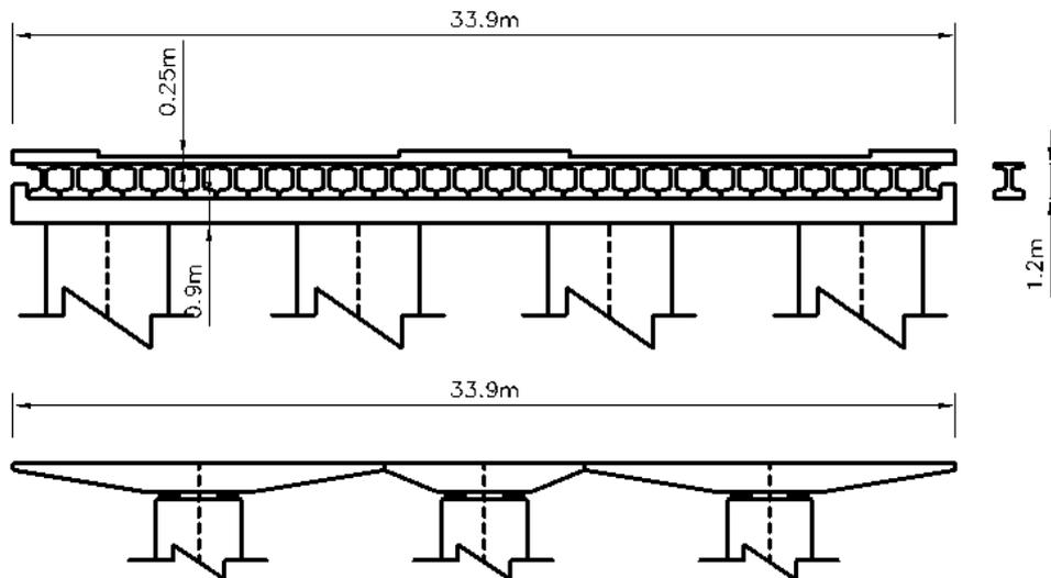
Figure 6. Kayabaşı Viaduct: Pre-tensioned Precast and Post-tensioned alternative.
