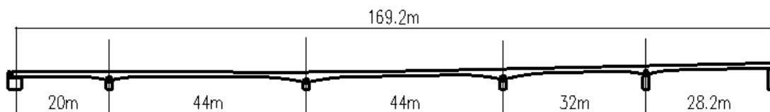
Figure 11. South-west approach viaduct at Haliç Metro Access Bridge.
