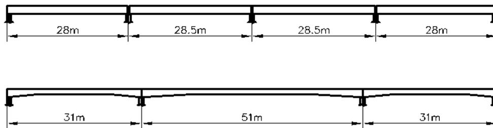
Figure 3. Span length comparison of simply supported and continuous systems.
