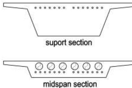
Figure 8. Variable cross-section at support and midspan (with voids).
