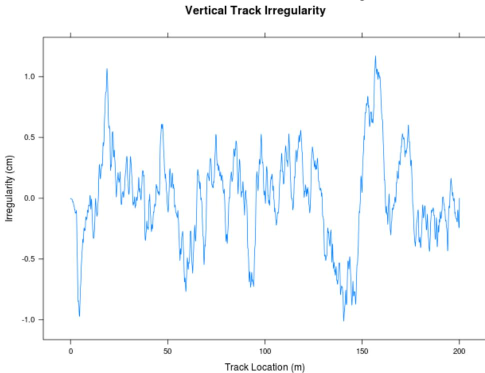
**Figure 3. Vertical track irregularity profile**
