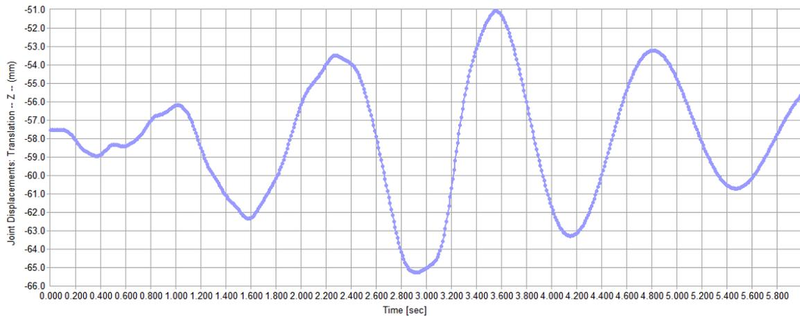
**Figure 4. Vertical displacement at the center of the front car as a function of time. Although the cars have left the track at 4.51 sec, the vehicle remains a part of the analysis until the final time step with wheels assumed to have zero displacement.**
