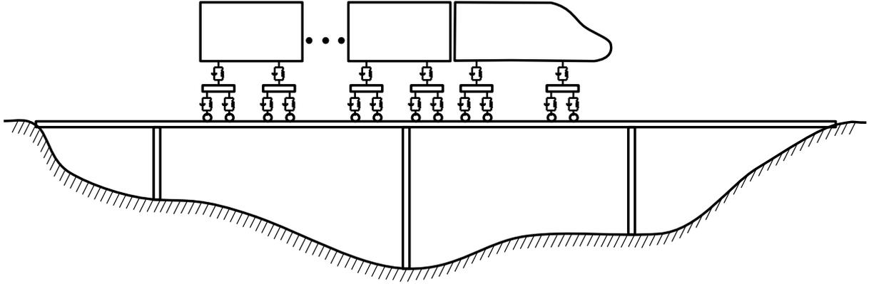
**Figure 1. Conceptual model of train traversing a bridge**
