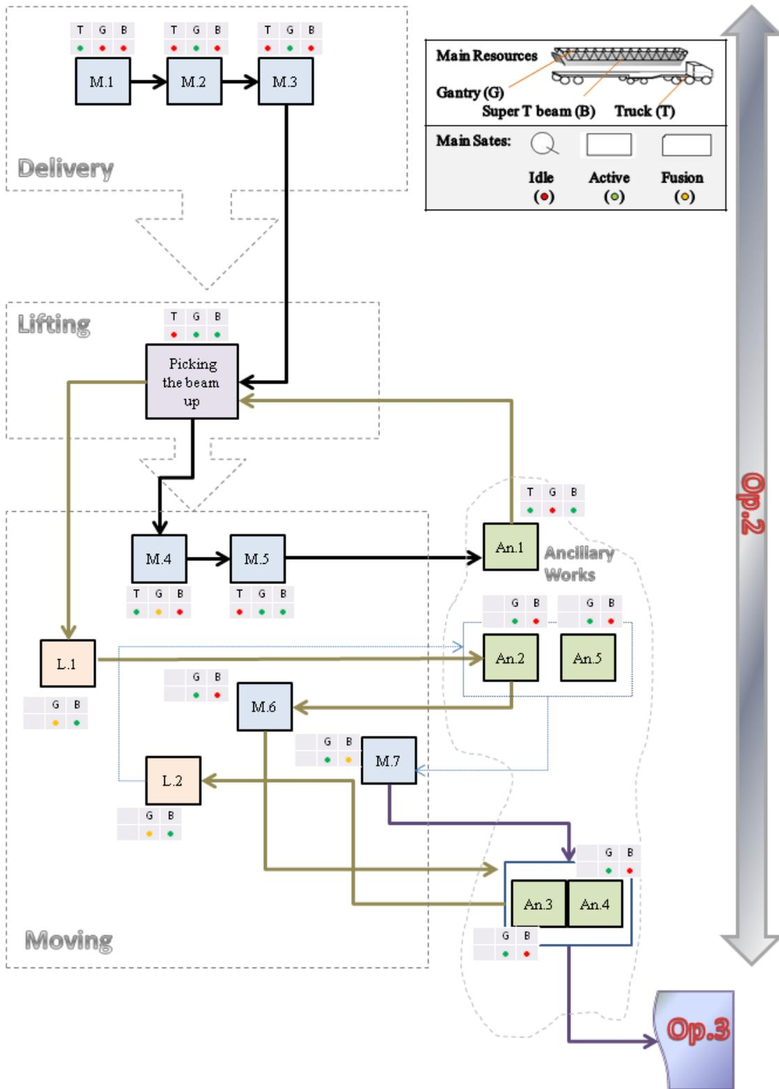
Figure 2. Conceptual model of installation operation of precast T-beams
