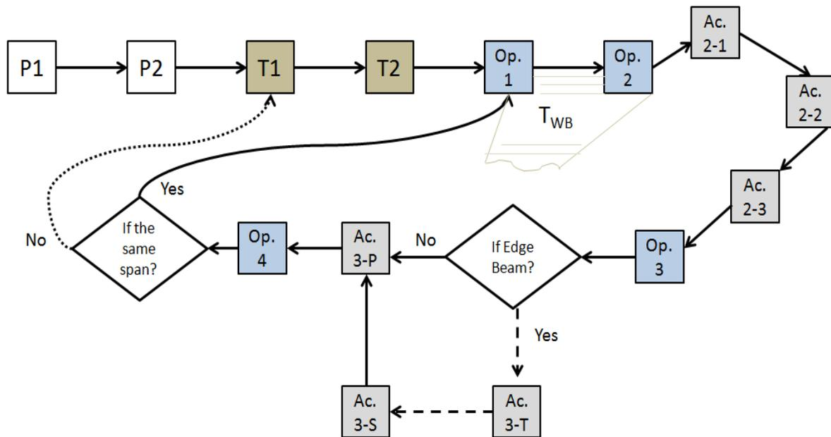
Figure 1. Conceptual model of bridge construction project using launching girder
