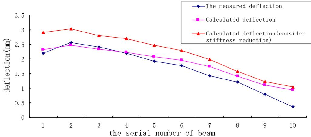
Figure 8. Comparison of the measured deflection and theoretical values at mid-span along transverse direction of bridge
