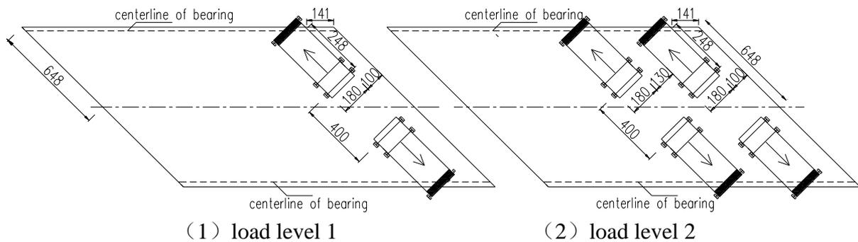
Figure 6. Loading position for bending moment in mid-span (Dimension. unit: cm)
