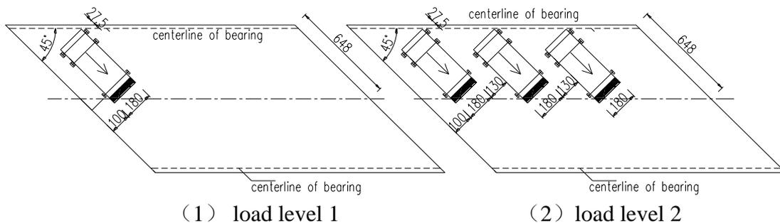
Figure 7. Loading position of shear force near the bearing (Dimension unit: cm)
