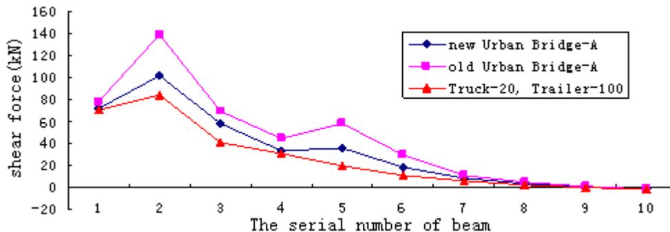
Figure 5. Shear force of the beams under different design loads
