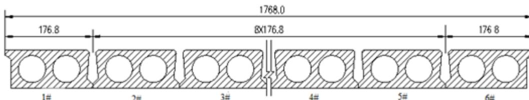
Figure 2. Cross-section of Xiazheyang Bridge
