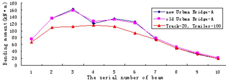
Figure 4. Bending moments at mid-span under different design loads
