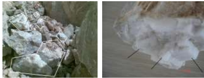
Figure 8, 9. Crystalline calcite rocks mixed in limestone after explosion.
