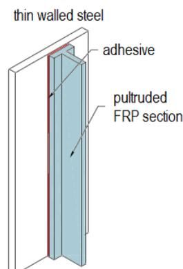
Fig. 1 Schematic representation of SBS method
