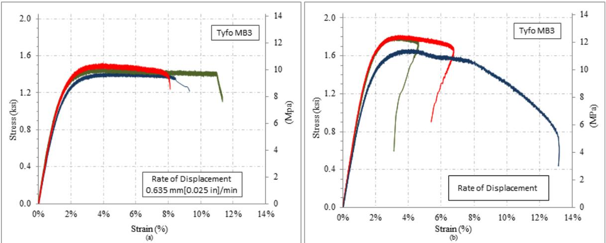
(a) 0.635 mm/min [0.025 in/min] strain rate      (b) 1.27 mm/min [0.05 in/min] strain rate
