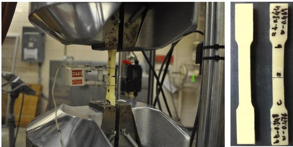
Fig. 2 Uniaxial tension test setup and epoxy coupons before and after the tension test
