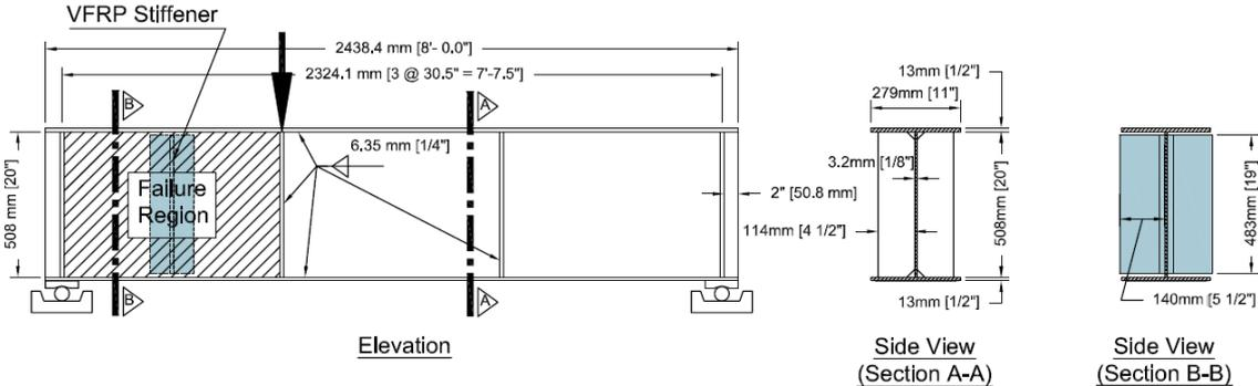
Fig. 3 Built-up I shape steel beams
