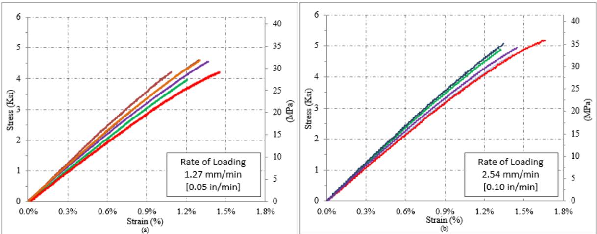
(a) 1.27 mm/min [0.05 in/min] strain rate      (b) 2.54 mm/min [0.10 in/min] strain rate
