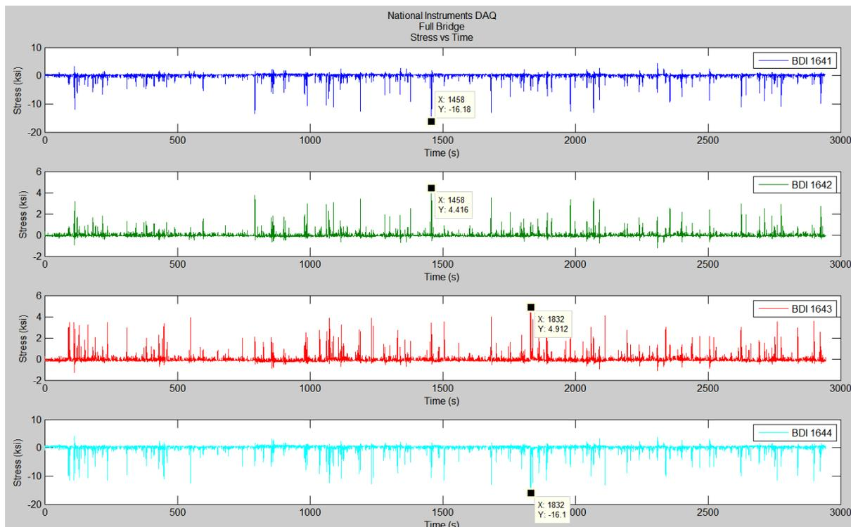
Figure 6. BDI strain transducer connection plate measurements. (Positive indicates compression; BDI1641 on G3 cracked side; BDI-1642 on G3 uncracked side, BDI-1643 on G4 cracked side and BDI 1644 G4 uncracked side)
