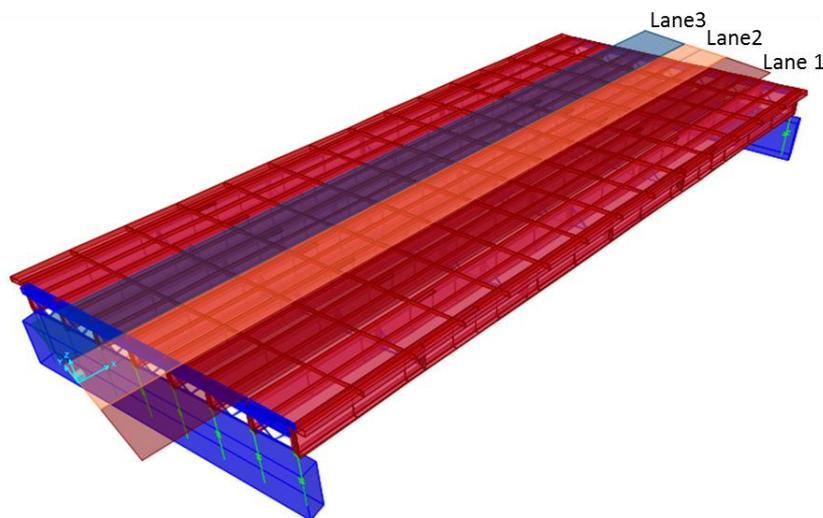
Figure 7. Finite element model with traffic lanes
