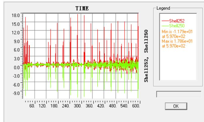
Figure 8. Vertical stress at lower end of connection plate (shell252-G3cracked side, shell250-G3uncracked side), unit-ksi.
