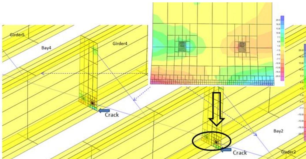
Figure 9. Zoom-in vertical stress contour of connection plate (Girder 3 Diaphragm 3) at T=597second
