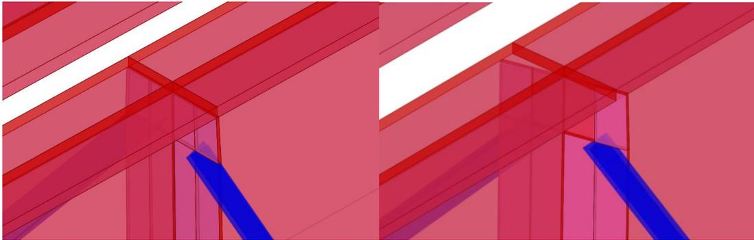
Figure 10. Skew (right) and non-skew (left) connection plates
