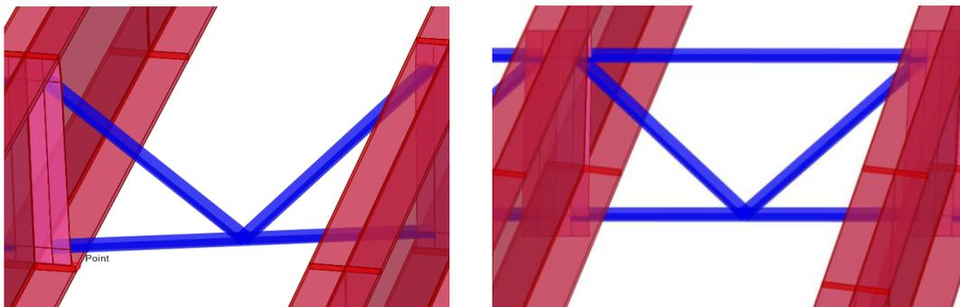
Figure 11. K-frame without top chord (left) and K-frame with top chord (right)
