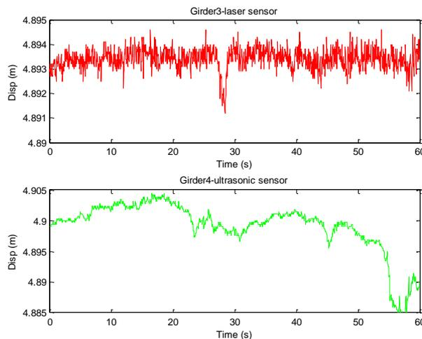
Figure 4. Bridge deflection data by laser sensor (upper) and ultrasonic sensor (lower). (The measured value is the distance between the sensor and girder bottom surface)
