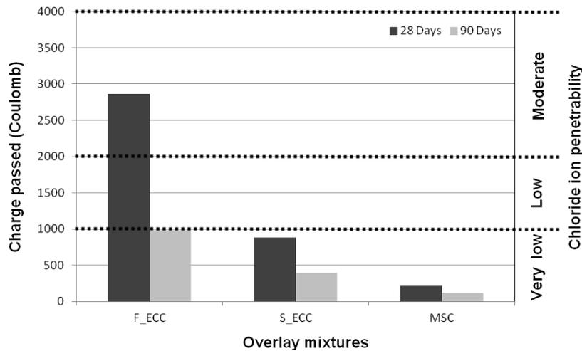
Figure 4. Chloride ion penetrability of overlay mixtures with charge passed.
