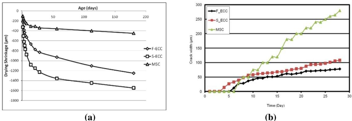
Figure 3. a) Drying shrinkages of overlay mixtures b) Crack width-time relations of overlay mixtures under restrained shrinkage.
