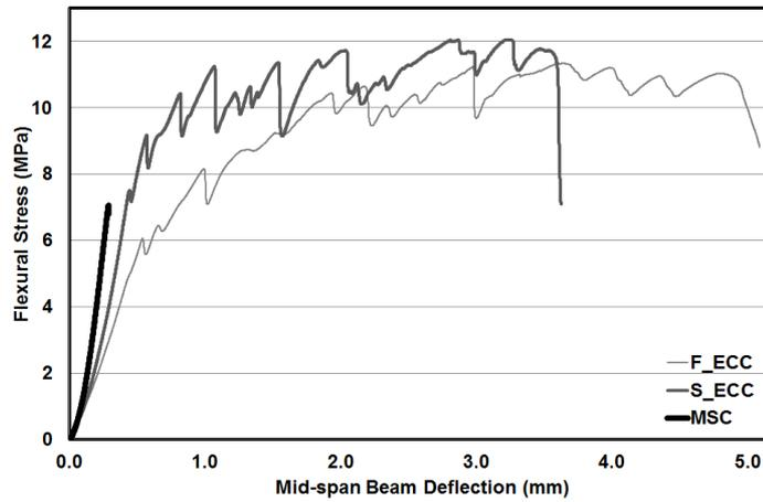
Figure 2. Flexural strength – mid-span beam deflection curve of overlay materials at 28 days of age.
