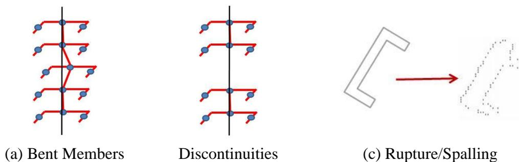
Figure 2. (a) Skeleton of a bent member, (b) skeleton of a discontinuous member and (c) modal and point cloud section cut of a C-section.
