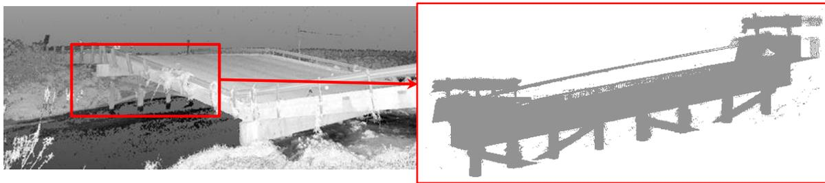
Figure 1: Point cloud of the entire DeKalb County Bridge and the processed portion of the dataset.
