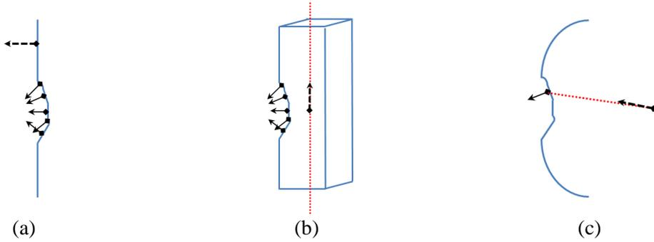
Figure 3. The representations of the reference normal and the normals from defect area: (a) from surface data, (b) from object with a skeleton and (c) from a surface with a reference point.
