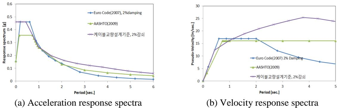
Figure 1. Response spectra according to the design code of each country.
