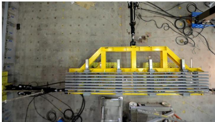
Figure 4. Seismic simulation test of expansion joint.
