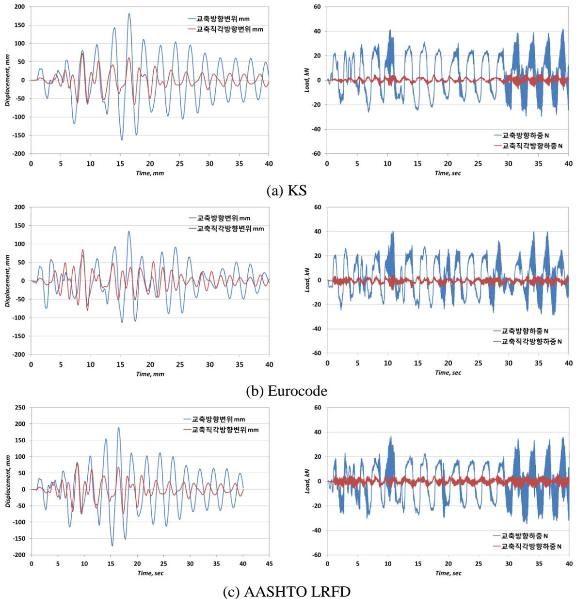
Figure 5. Time histories of displacement and load according to each design code.
