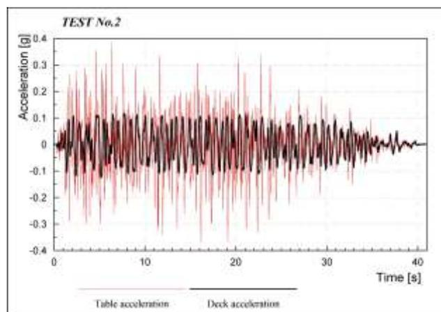
Figure 10. Time histories of table and deck accelerations. Test #2
