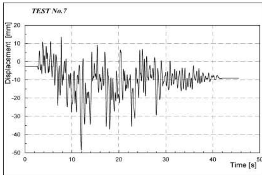
Figure 11. Time history of displacement of the tapered pin. Test # 7.
