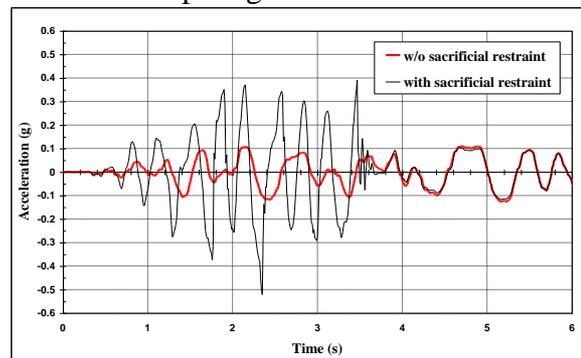
Figure 9. Time history of deck acceleration. Comparison of tests #1 and #2
