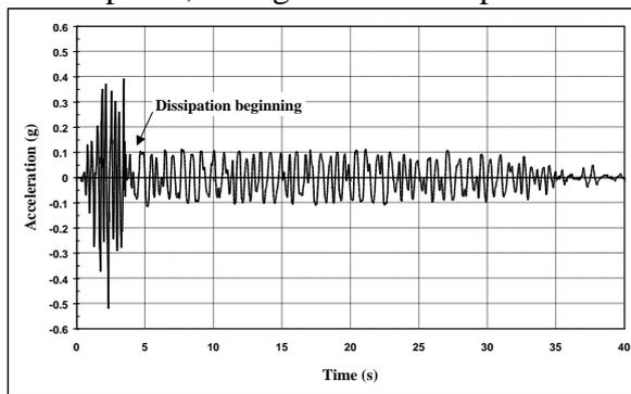
Figure 8. Time history of deck acceleration. Test with sacrificial restraint.
