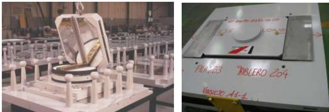
Figure 2. Isolators in workshop (left during assembling phase – right as assembled) (type positions 2 and 3 of figure 1)
