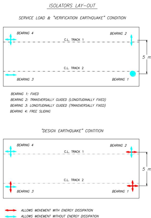
Figure 1. Typical isolators lay-out.
