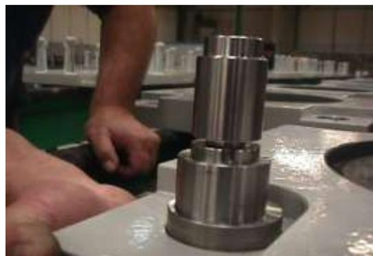
Figure 4. Installation of a sacrificial element.
