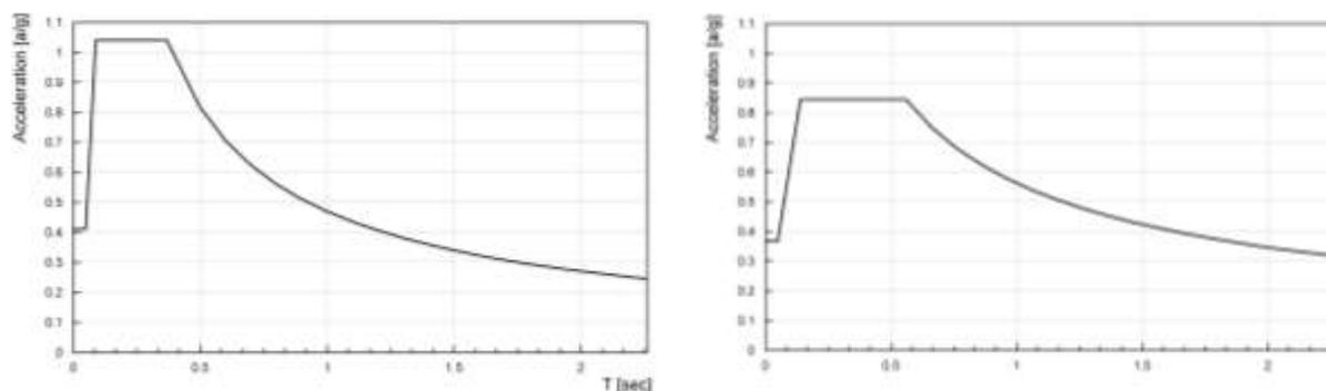
Figure 7 - Design acceleration spectrum type AST (left) and type IMP (right).
