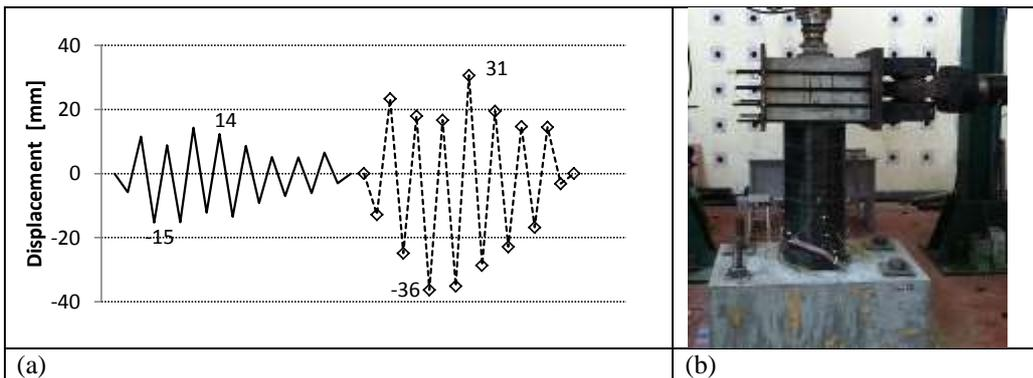
Figure 5 Cyclic test on pier specimens: a) Displacements histories applied on top pier specimens during the first (PD1, Tolmezzo; continuous line) and the second (PD2, Tolmezzo x 2; dashed line) cyclic tests; b) test apparatus.
