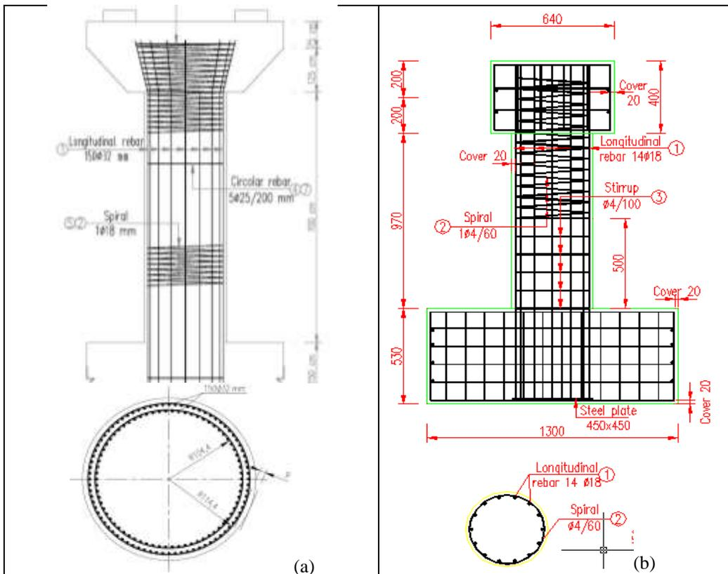
Figure 3 Chinese rc bridge: a) most stressed pier geometries and longitudinal and transversal steel reinforcements; b) pier specimen (scale 1:6) geometries and longitudinal and transversal steel reinforcements.
