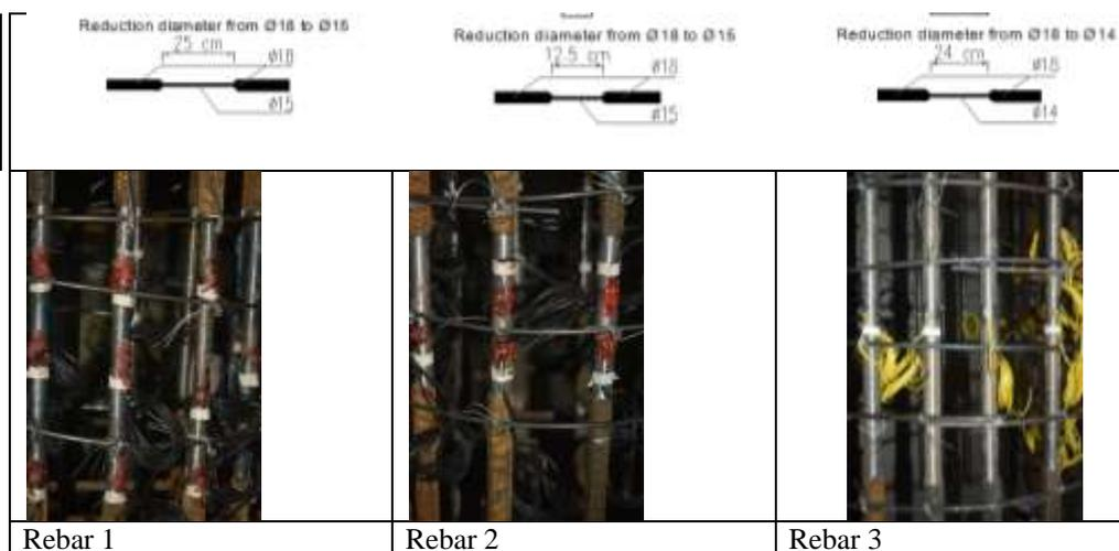
Figure 4 Chinese pier specimens with turned rebars: three different (Rebar 1, Rebar 2 and Rebar 3) longitudinal turned rebar configurations
