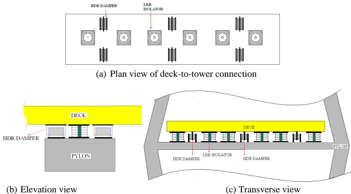
Figure. 2. Overview of the hybrid control system applied in deck-to-tower connection
