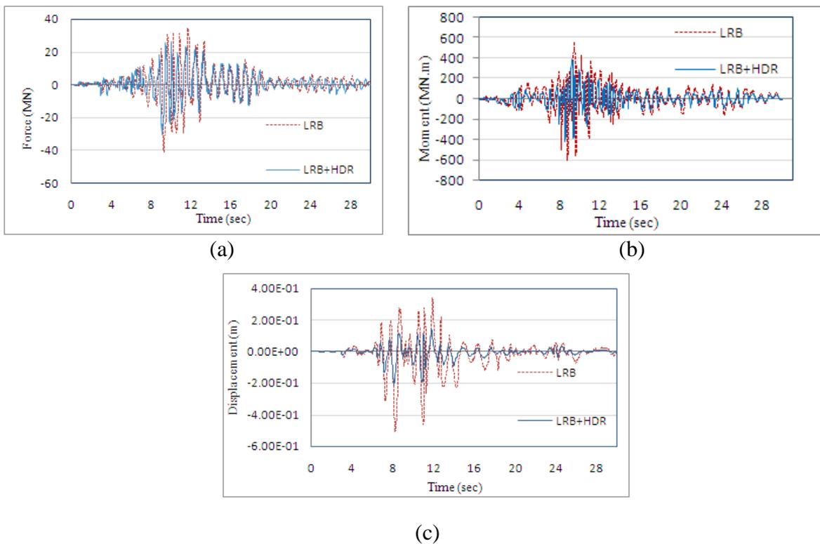
Figure. 3. (a) Base shear force, (b) Base moment and (c) Deck displacement time history responses of the controlled cable-stayed bridge using LRB+HDR compared to the controlled bridge using LRB (Kobe 1995) ( $\xi=0.18$ )
