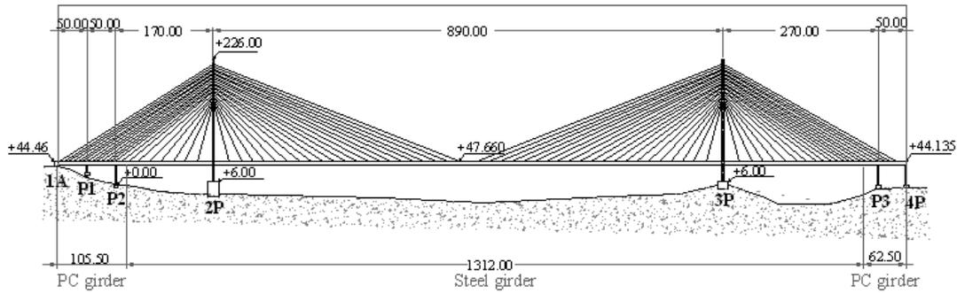
Figure. 1. General arrangement of the Tatara cable-stayed bridge
