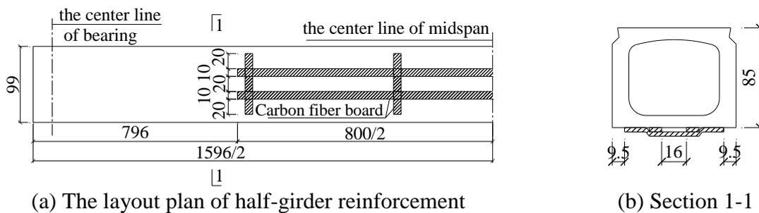
Figure.13 Schemes of girder reinforcement (unit: cm)
