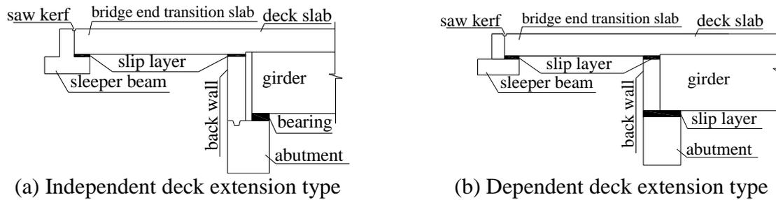
Figure.10 Jointless bridges with deck extension
