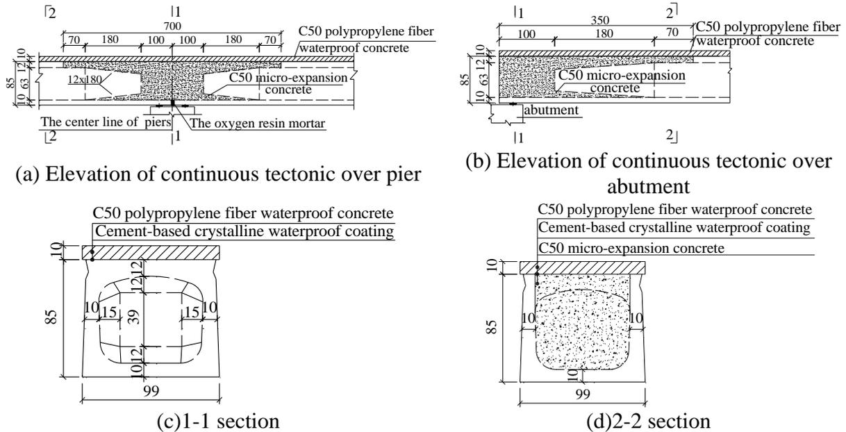
Figure.11. Simply-supported to continuous structure system (unit: cm)
