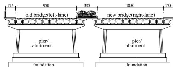
Figure. 2 Cross-section (unit: cm)
