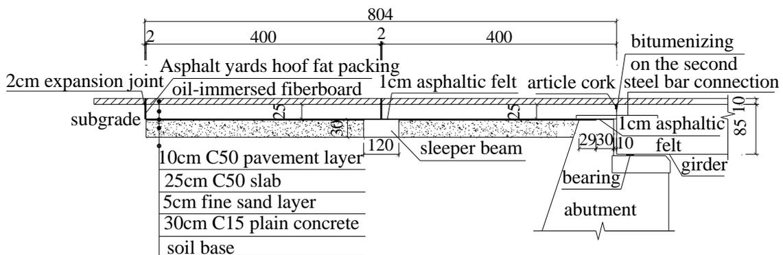
Figure.14. Elevation of jointless abutment (unit:cm)
