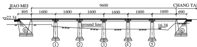
Figure. 1 Elevation layout (unit: cm)
