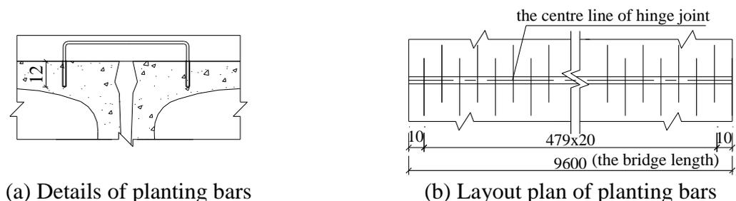
Figure.12 Schematic diagram of connection between the cast-in-place deck pavement and the original structure (unit: cm)
