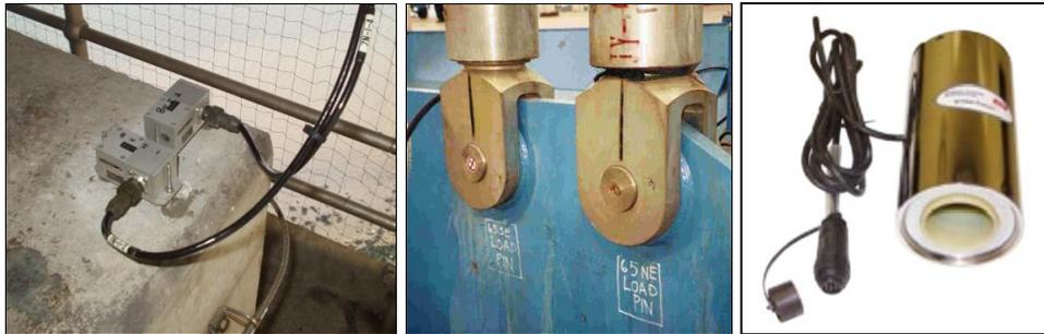
Figure 5. (Left to right): Inclinometers, load pin and magneto-elastic sensor.
