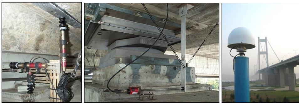
Figure 4. (Left to right): Typical linear variable displacement transducers, magnetostrictive sensor, and GPS/GNSS receiver.
