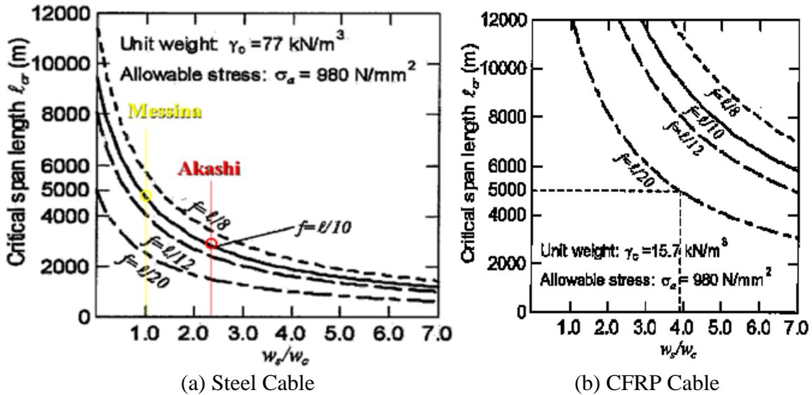
Figure 2. Critical span length for steel (a) and CFRP (b) cables.
