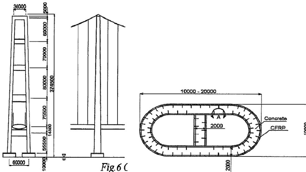
Figure 5. Cross section of the tower.
