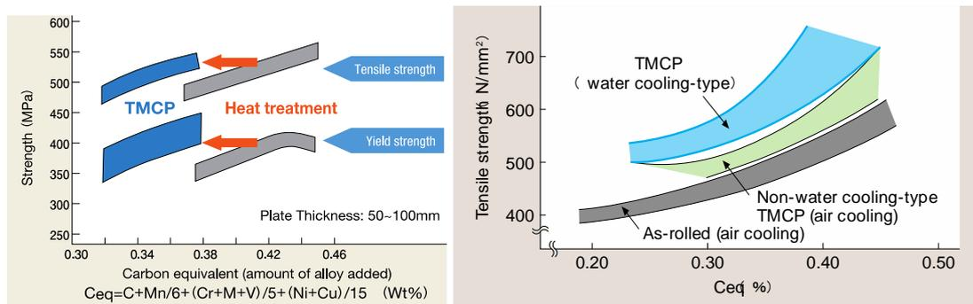
Figure 6. The effect of TMCP and comparison with conventional manufacturing process [7]
