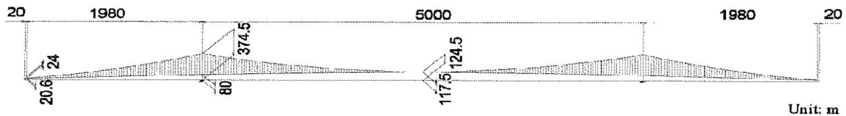
Figure 3. General view of the 5000m span suspension bridge.
