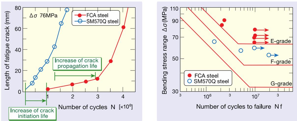
Figure 8. Comparison of fatigue strength of FCA and conventional steel.
