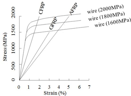
Figure 1. Comparison of CFRP wire with steel wire.
