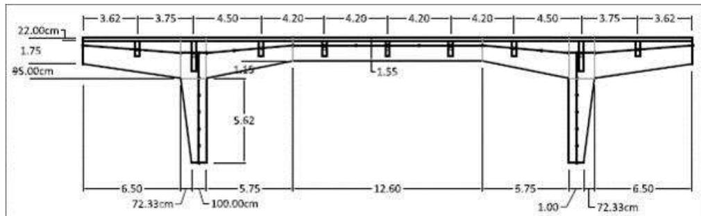
Figure 1.2. The longitudinal section of the structure
