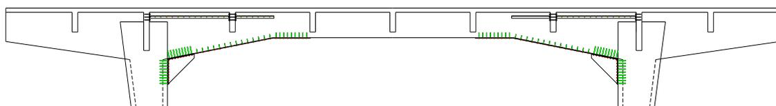
Figure 5.2. General view of strengthening of existing column-beam connections and of beams by additional steel plates.
