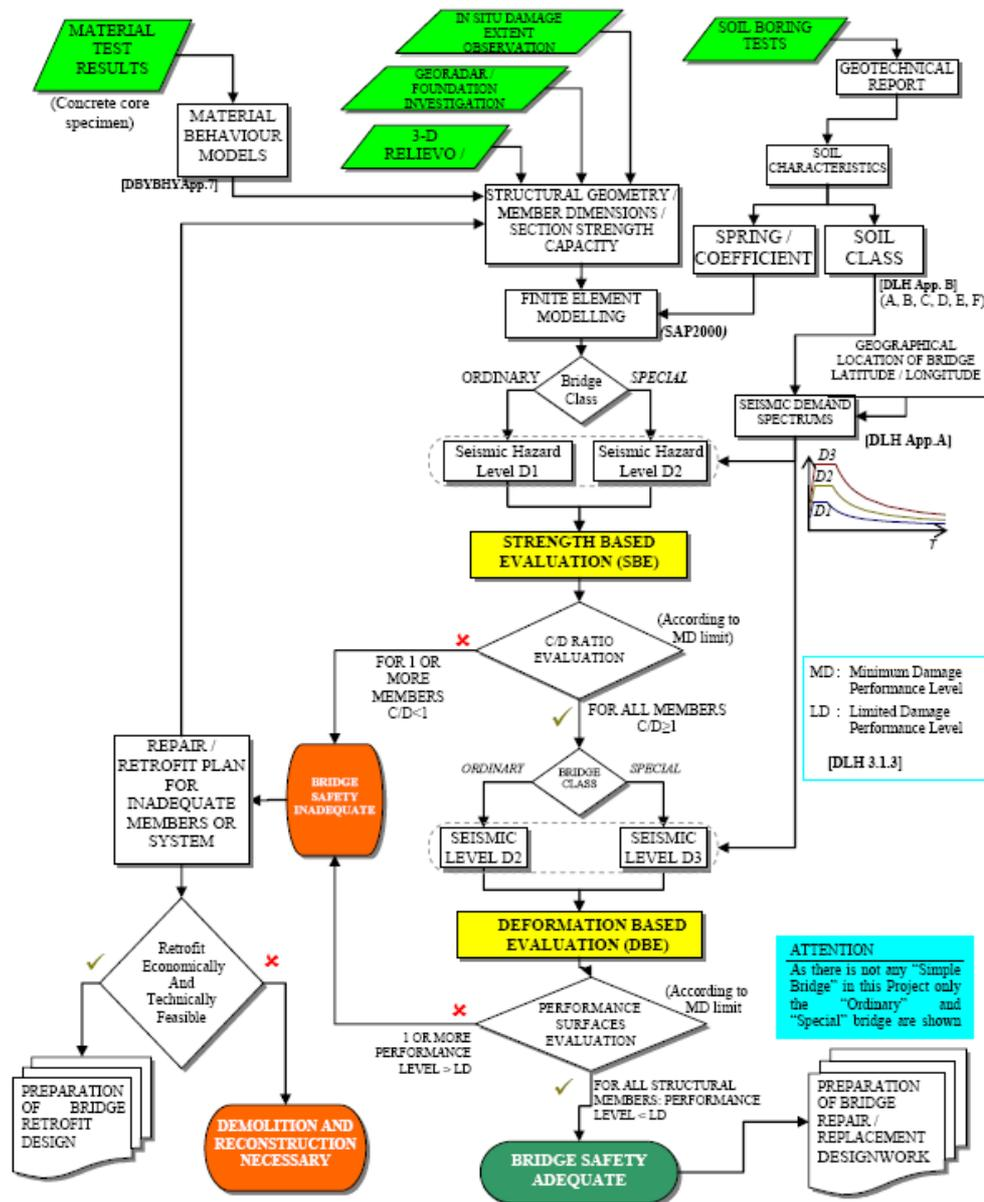
Figure 3.2. Flowchart relating to seismic performance evaluation of bridges
