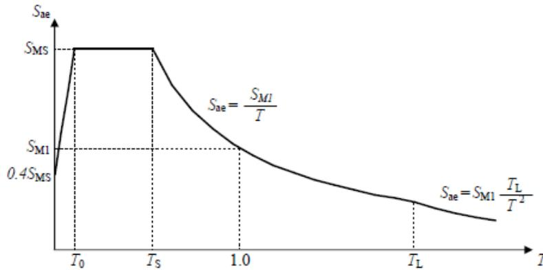
Figure 3.1. Seismic design response spectrum [DLH 1.2.2.1 & 1.2.2.2]
