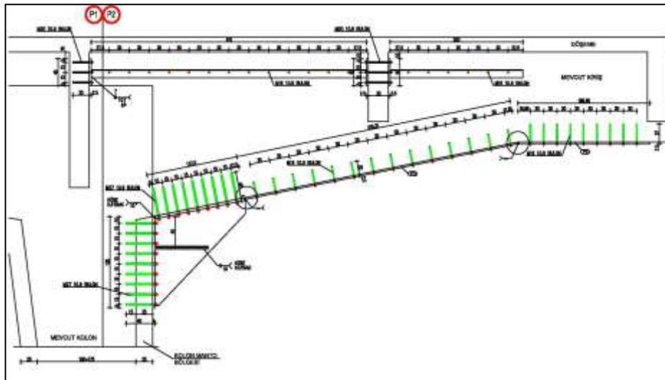
Figure 5.3. Strengthening of existing column-beam connections and of beams by additional steel plates.
