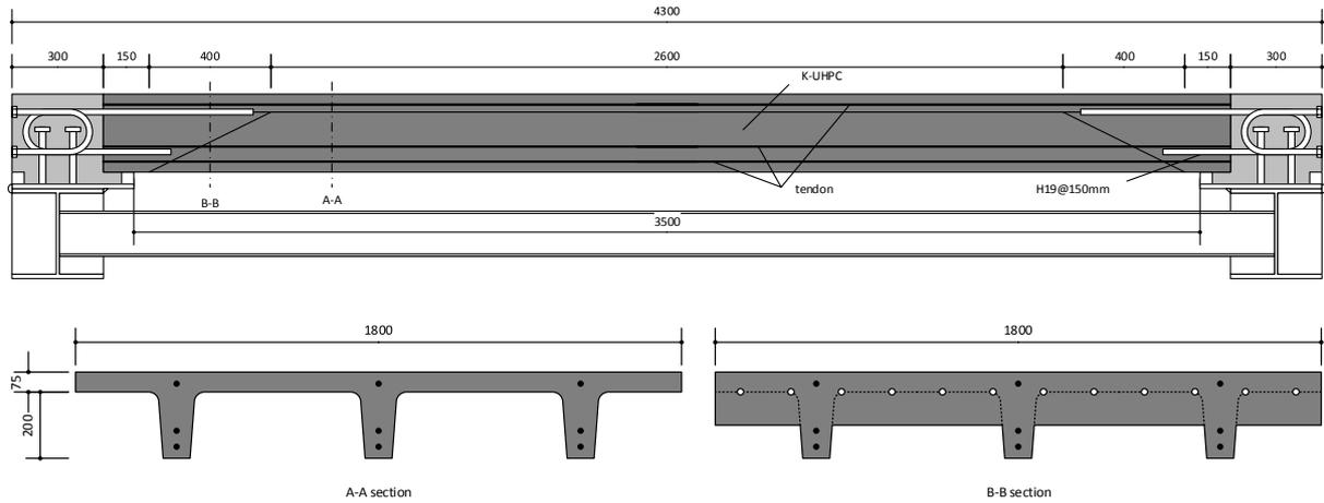
Figure 2. Shape and dimensions of specimen.
