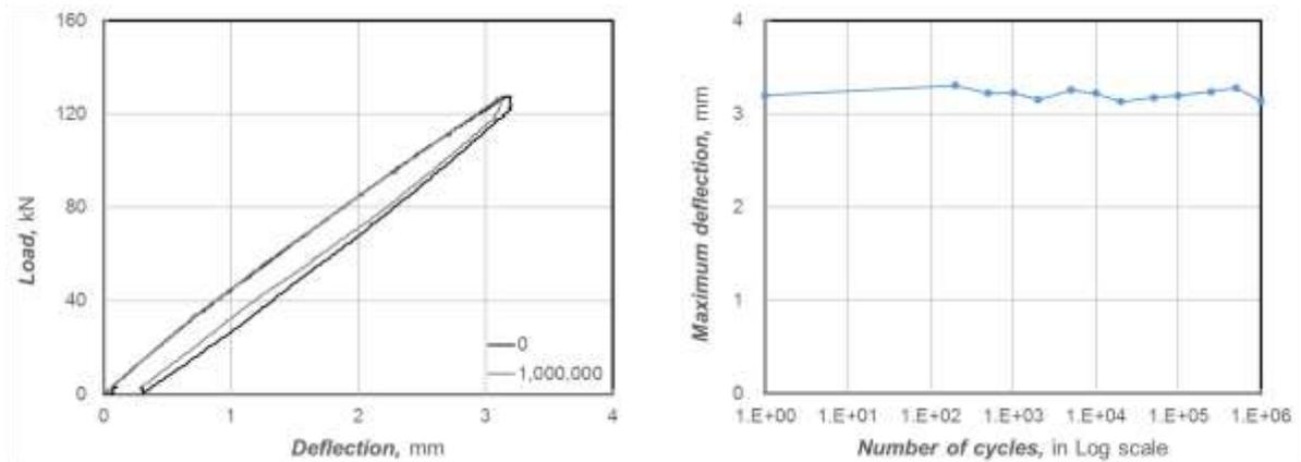
(a) Comparison of load-deflection curves at initial stage and after 1 million cycles
