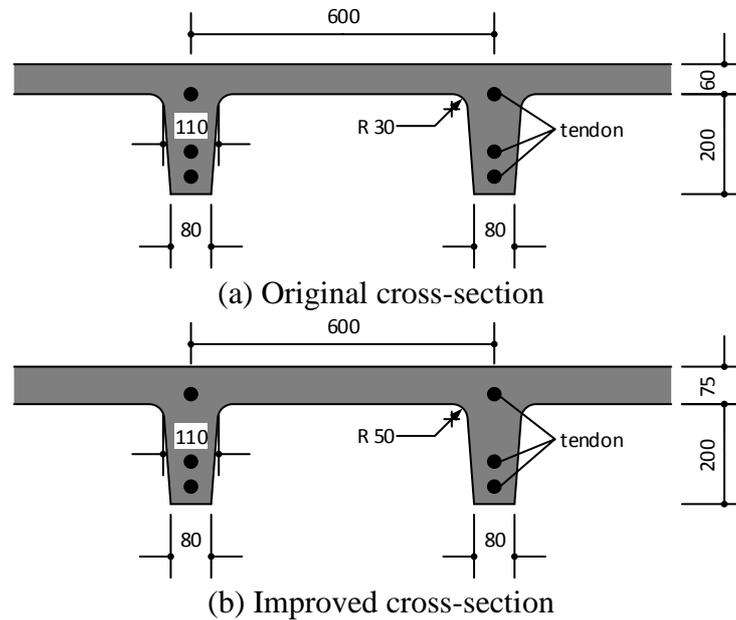
Figure 1. Improvement of the cross-section of UHPC rib-type deck.
