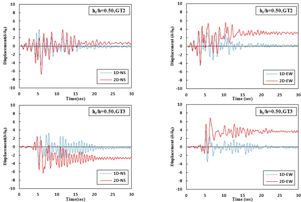
Figure 5. Displacement response of test specimens.
