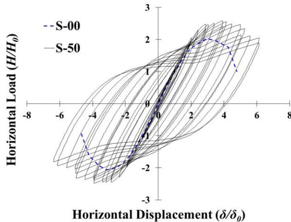
Figure 3. Hysteresis curves for static cyclic loading tests.
