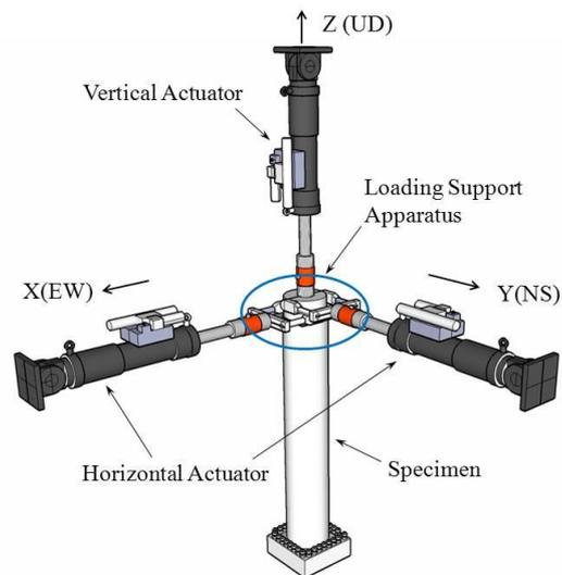
Figure 2. 3D loading system.
