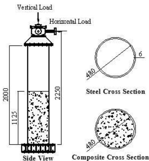
Figure 1. PCFST specimen used in the test (unit: mm).
