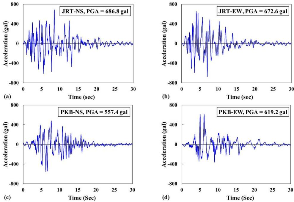
Figure 4. Input earthquake components used for hybrid loading test.
