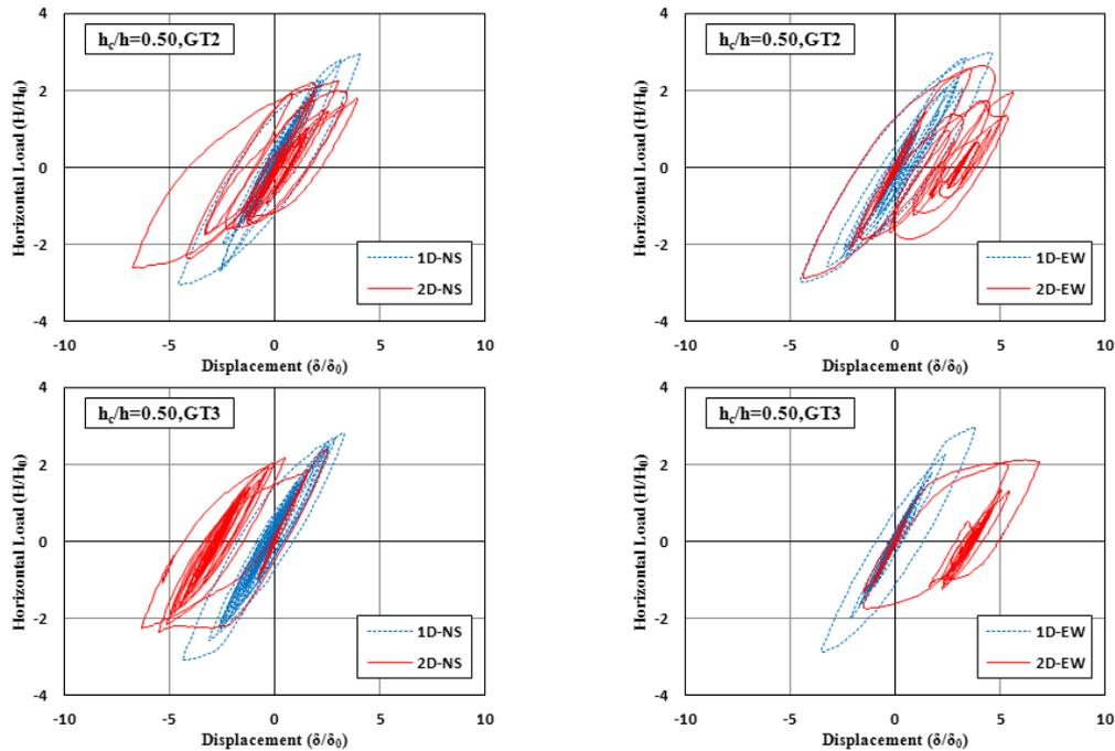
Figure 6. Hysteresis curves of test specimens.
