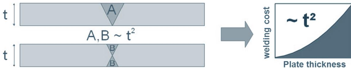
Figure 5. Realizable cost savings in welding dependent on plate thickness
