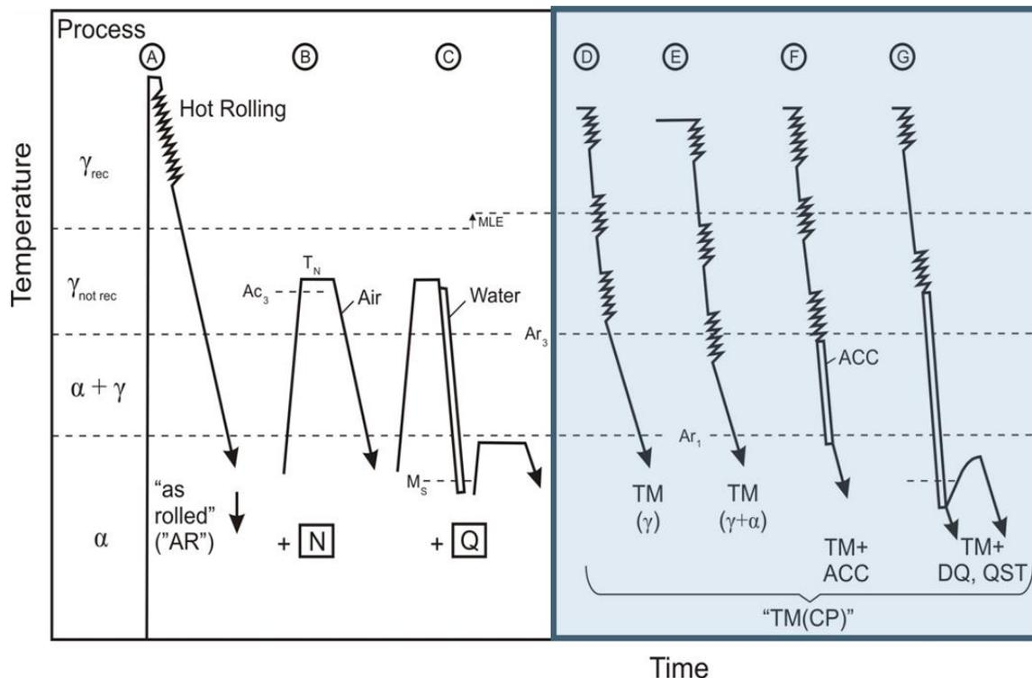
Figure 1. Schematic temperature-time-procedures used in heavy plate production [3]
