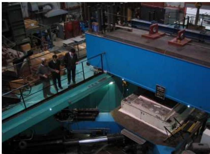
Figure 11. HL MDB undergoing testing at SRMD test facility.
