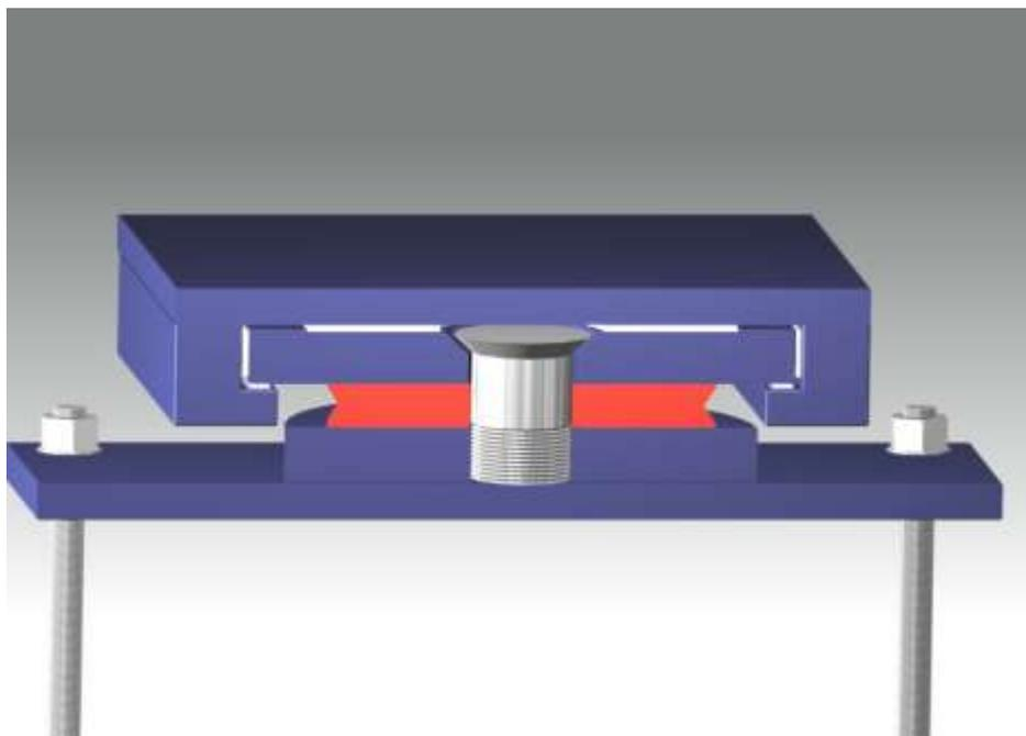
Figure 9. Uplift restraint HLMDB.
