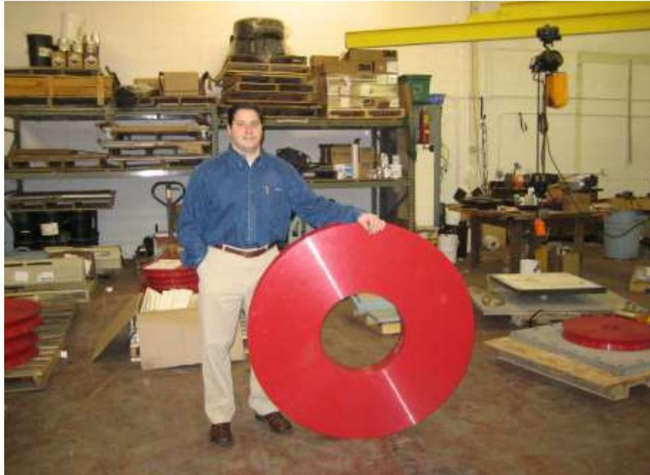
Figure 8. Polyurethane rotational element for a 25,780 kN HLMDB.
