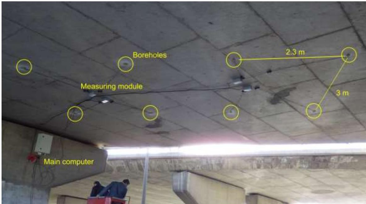
Figure 6. Installed monitoring system at Izmir – Aydin Bridge, Turkey, with boreholes and data acquisition nodes.
