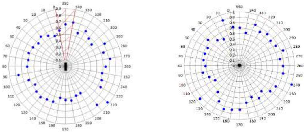
Figure 3. Directional characteristics of the sensor parallel (left) and perpendicular (right) to its symmetry axis. No representative amplitudes could be taken between 340° and 360°, because of the position of the sensors cable.
