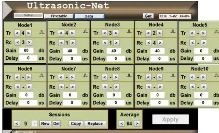
Figure 8. Web based configuration panel to set transmitter/receiver combinations and the signals amplification.
