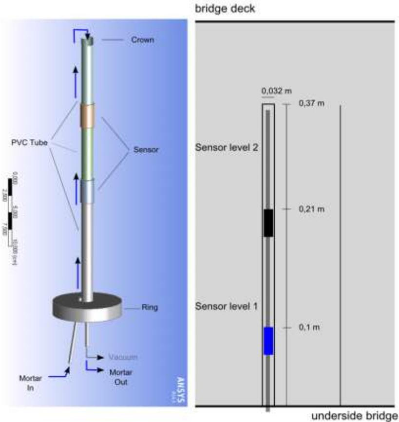
Figure 5. left: Sketch of the mortar injection into the borehole. Right: Two levels of sensors in depths of 10 cm and 21 cm.
