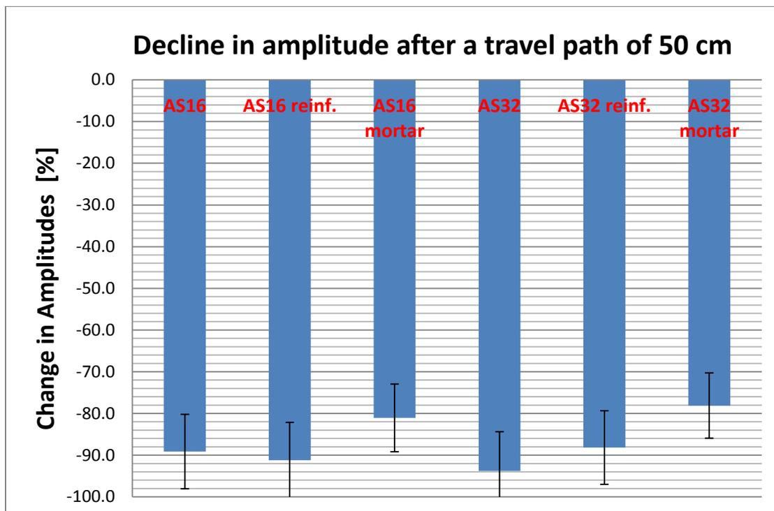
Figure 4. Attenuation of signal amplitudes depending on aggregate size, reinforcement and different methods of embedding the sensors.
