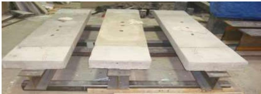
Figure 5. Link slab specimens after casting
