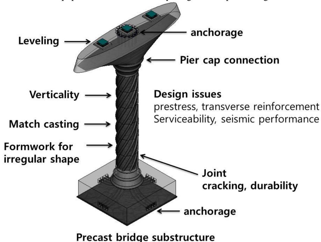
Figure 1. Design and construction issues of a precast bridge pier
