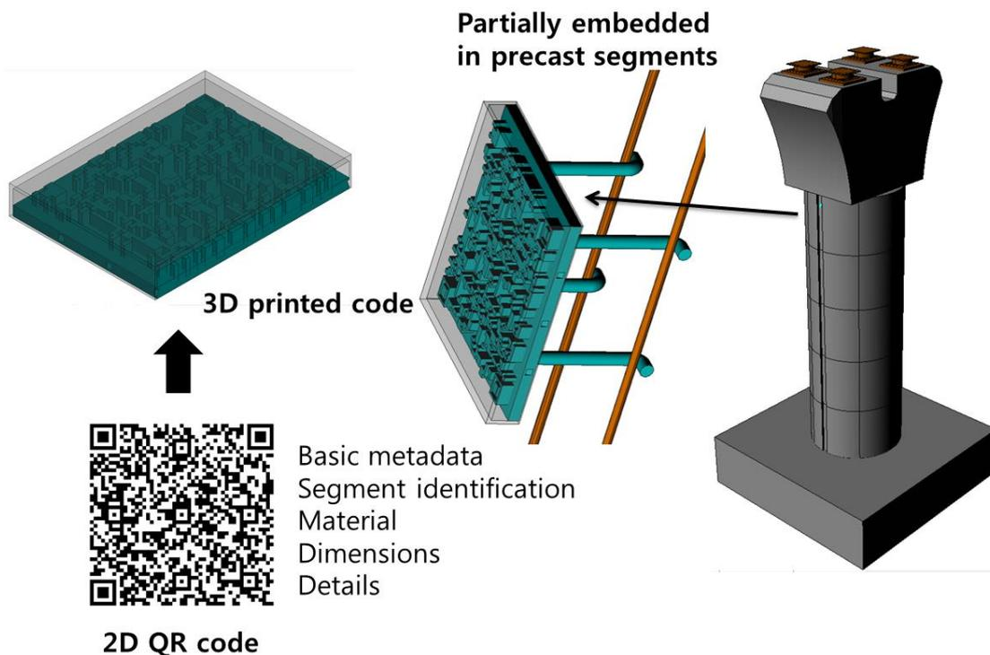
Figure 3. 3D printed QR codes
