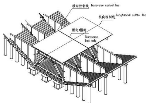
Figure 7. Box girder fabrication
