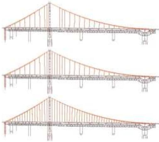
Figure 16. Three phases of load transfer via hanger installation
