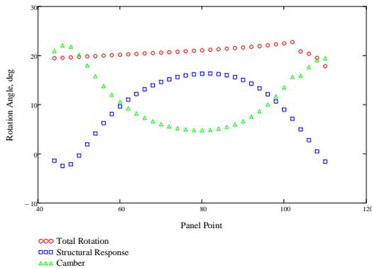
Figure 18. Cable twist and camber
