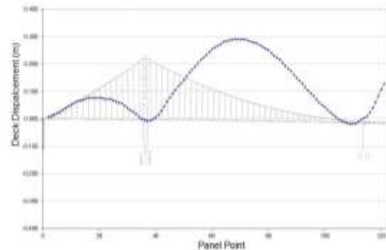
Figure 17. Deflection of box girder after phase 1 of load transfer
