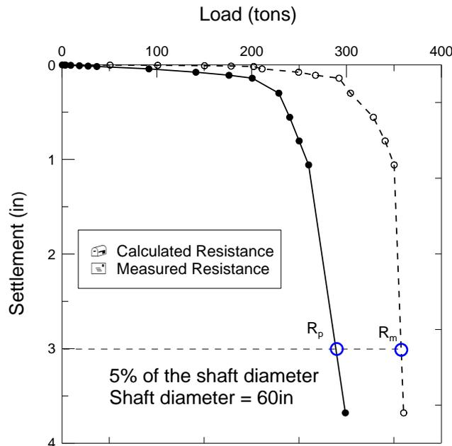
Figure 4. Example of load-settlement analysis and measured value.
