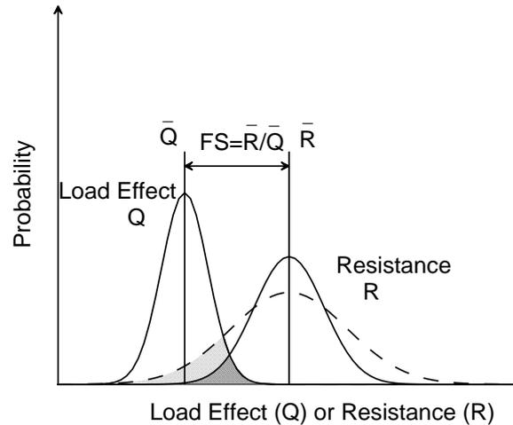
**Figure 1.** Probability density functions for structure load and resistance.
