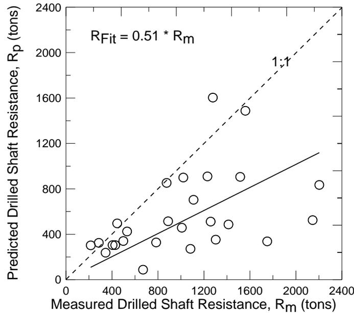
Figure 5. Measured ( $R_m$ ) versus predicted ( $R_p$ ) drilled shaft resistance.
