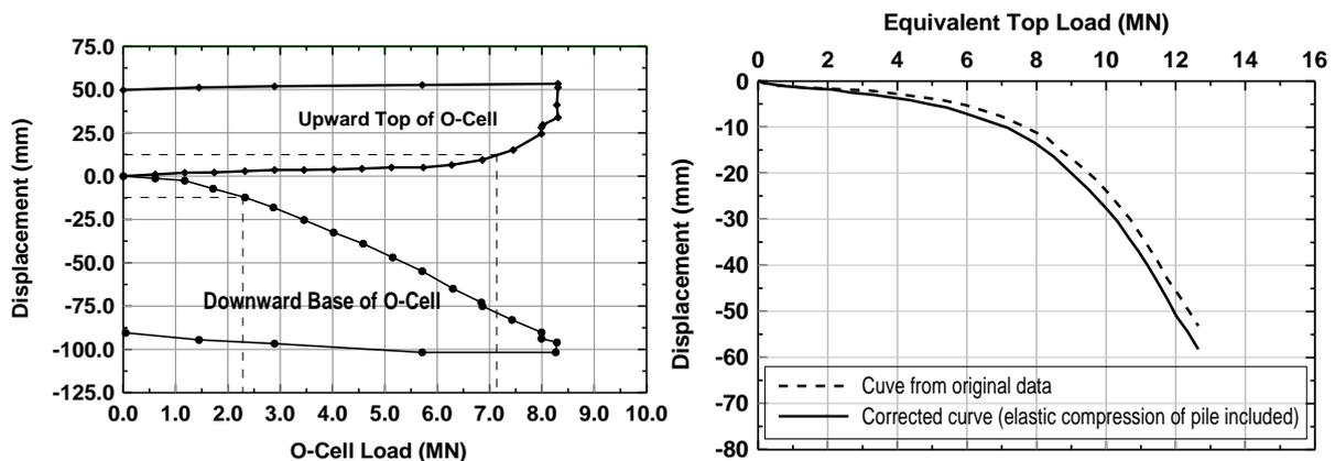
Figure 3. a) Settlement curves by O-cell b) equivalent top-down settlement curve.
